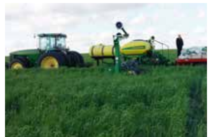
Soybeans are planted into a cereal rye cover crop. The no-till planter has helpful “bells and whistles” such as row cleaners, seed firmers, pneumatic down pressure and drag chains.
