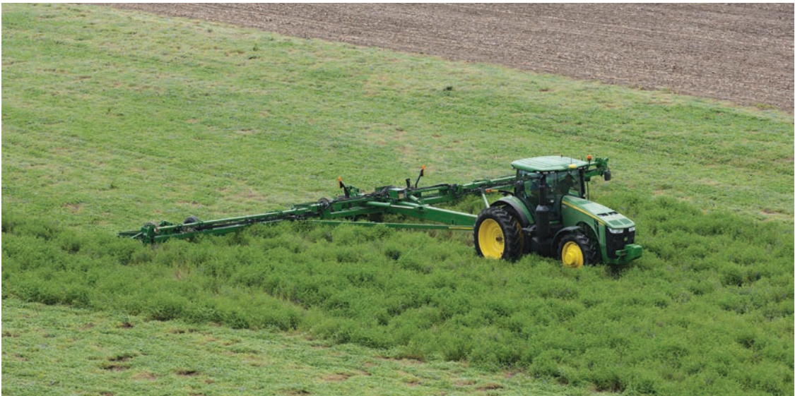
This custom-built 60-foot roller crimper helps to manage cover crops on commercial scale research farms. We believe this is the largest roller crimper in the world, designed on a John Deere 1770 NT tool bar to match up with a 24-row 1770 NT planter and to fold to 12-feet wide for transportation.
